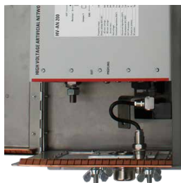
Full screening using screened room door technology
